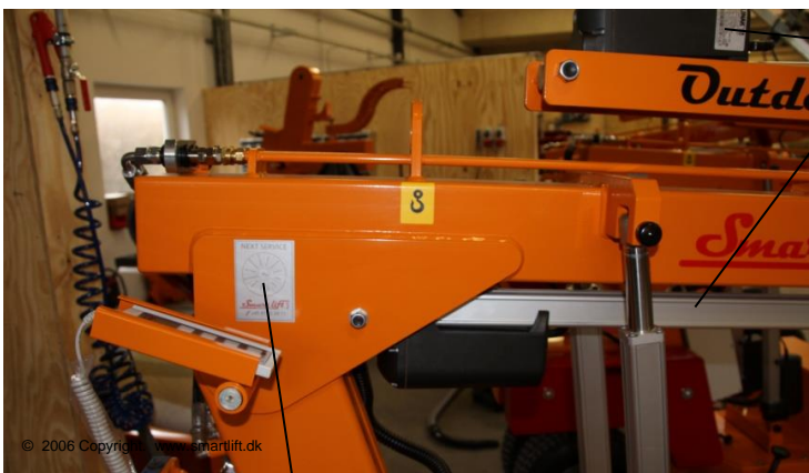
Service sticker – According to legislation SL-OUTDOOR must be serviced once a year
