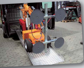
The compact Smartlift design allows for easy transport by van or trailer.
