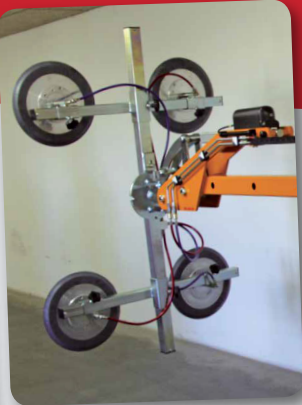
The yoke allows multidirectional movement.
