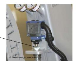
To re-establish function on the machine, you may, for instance, using a screwdriver push up the switch, and the safety switch will resume its function
