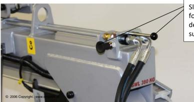
Slide Valve w/safety lock for activation and deactivation of vacuum suction.
