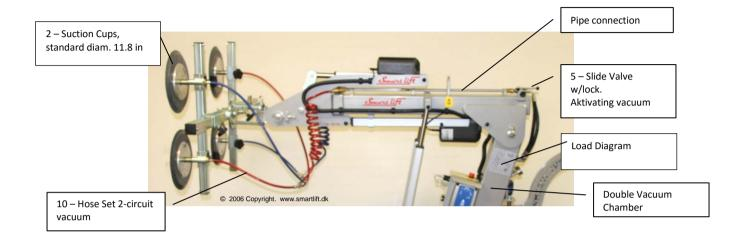
For max. stability at transport of sucked work, the suction cups are to be centred and adapted to the transport work chosen. *Operation of yoke with sucked work should <u>always</u> be conducted with caution*
