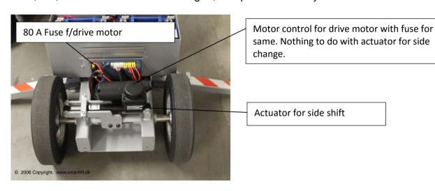
To check this actuator, remove the protective screen. In case of lacking or wrong function, check for any murmuring/noise and loose lines.
