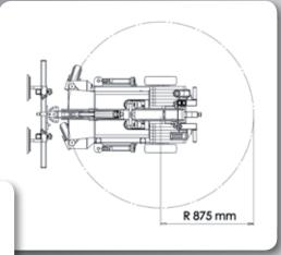
The two powerful 1500 W electric motors mean that the SL 208 Compact can rotate on its own axis. All it requires is a firm surface.
