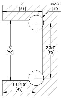
Cutouts provide 1/8-1/4" clearance between glass and wall
