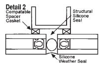
For insulating glass, the design must be changed to accommodate Figure 1 and Detail 2, unless a one component silicone secondary
